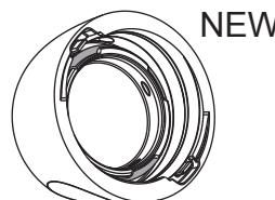
**⚠** Check the state of the threads of the powder chamber and cap. The powder chamber is pressurized during use. The condition of the powder chamber and cap is an important safety factor.
